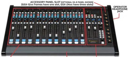
FADER CHANNELS (FOUR PER INPUT PANEL) PALM REST MASTER PANEL
