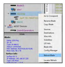
If the issues are still not resolved, then the Mix Engine and/or GSX Surface may need to be power cycled. This will cut off all audio thru the GSX console. Since neither the Mix Engine nor the PS-1600 Power Supply have power switches, their IEC AC cords will need to be unplugged from their AC outlets, or from the jacks on their rear panels. Wait ten seconds then reapply power to ensure all voltages are completely dissipated.
